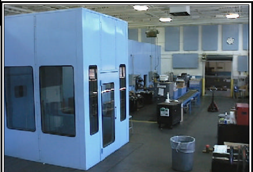
Rigid enclosure used in conjunction with wall absorbers
