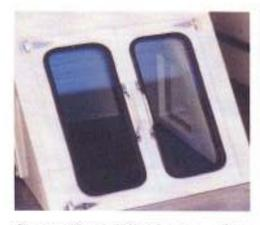
Acoustical Windows - Our standard windows incorporate double-paned, 1/4" thick laminated glass. The internal cavity is lined with acoustical foam. This design blocks noise through the two panes of glass and provides a more aesthetically-pleasing look.
