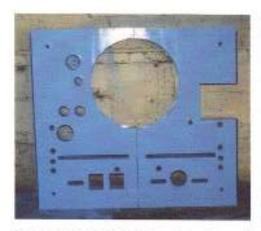
Custom Cut-Out Panels - Sound Barriers can customize panels to accommodate existing gauges, hoses, valves, conduit, etc. The tolerance of the above job was within 3/32 of an inch.
